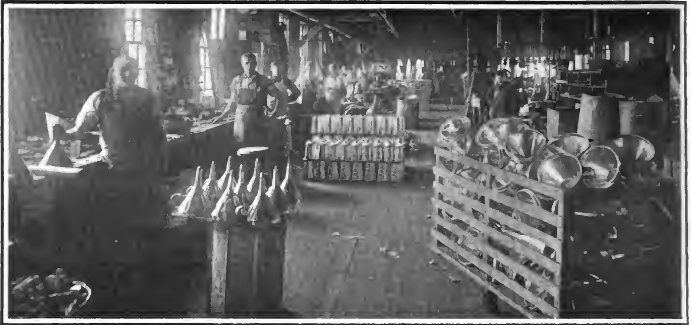
Finishing Room of the Dover Plant, Where Spouts and Handles Are Fitted to the Buckets and Funnels
